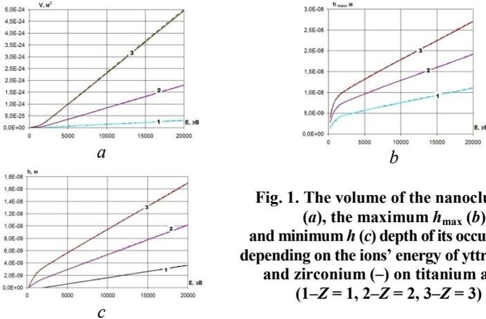
**Fig. 1. The volume of the nanocluster  $V$  (a), the maximum  $h_{\max}$  (b) and minimum  $h$  (c) depth of its occurrence depending on the ions' energy of yttrium (–) and zirconium (–) on titanium alloy (1– $Z = 1$ , 2– $Z = 2$ , 3– $Z = 3$ )**
