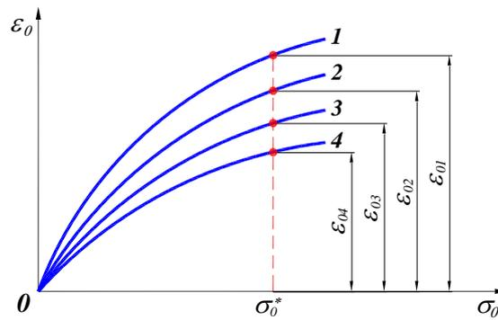
Fig. 3. Changing the volume deformation in tests with constant stress,  $\xi = \text{const}$
