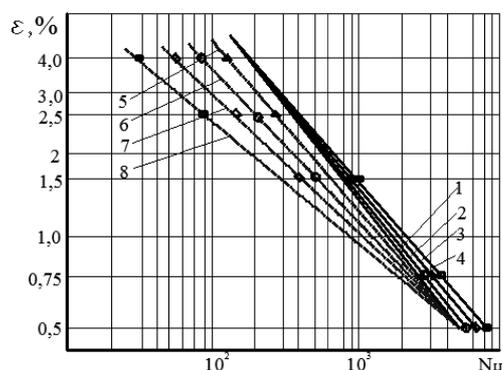
**Fig. 5 – Low-cycle durability of steel 40X**
