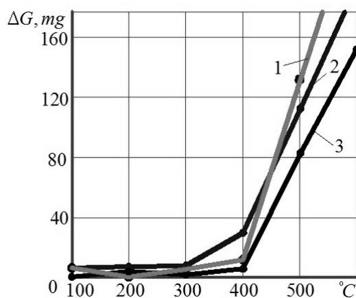
Fig. 2 – Dependence of mass losses in hydrosis of tempered steels from the temperature of release: 1 – steel 40; 2 – steel U12A; 3 – steel 40XN [5]
