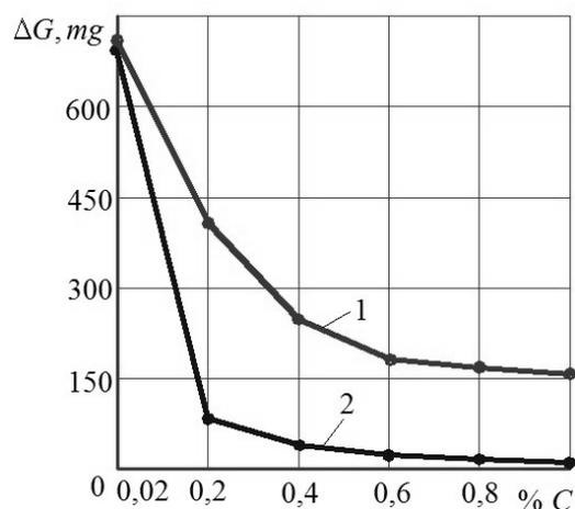
Fig. 1 – Hydrozoerosive wear resistance of carbon steels depending on the carbon content: 1 in annealed and 2-in tempered state [9]
