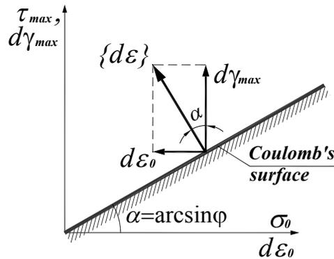
Fig. 7. The combination of stresses and strain rates
