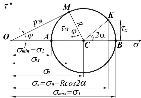
**Fig. 5. The limited circle of stresses by the Mohr - Coulomb condition**
