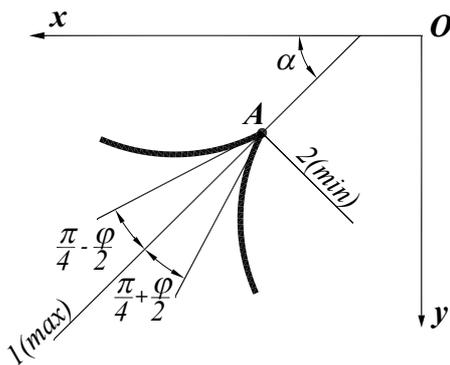
Fig. 6. Orientation of sliding lines
