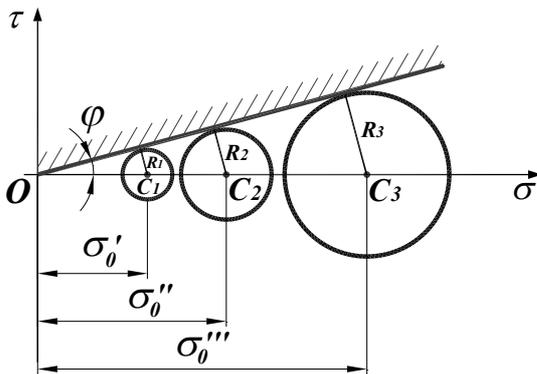
**Fig. 4. A family of Mohr circles describing the limited state of the discrete environment**
