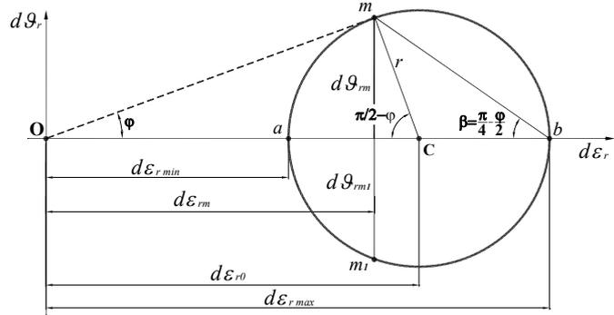
Fig. 9. Circle diagram  $d\vartheta_r - d\varepsilon_r$  of strain rates of discrete environment in the limited state
