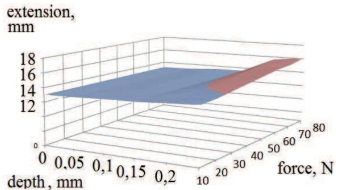
Fig. 11 Graph of stretch material with a certain thickness of the polymer coating on the strength of the load
