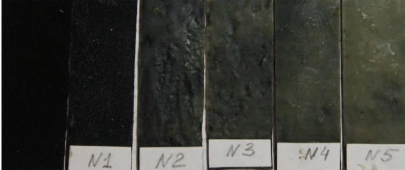
Fig. 5 Samples were coated with a polymer coating of varying thickness
