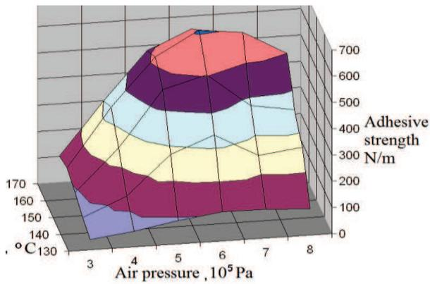
Fig. 8 Dependency of adhesive strength of polymer on temperature ( $^{\circ}\text{C}$ ) and pressure air spray ( $10^5\text{Pa}$ )
