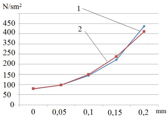
Fig. 10 Effect of thickness of the polymer film of conditional flexural stiffness (1 - experimental data 2 - theoretical data)
